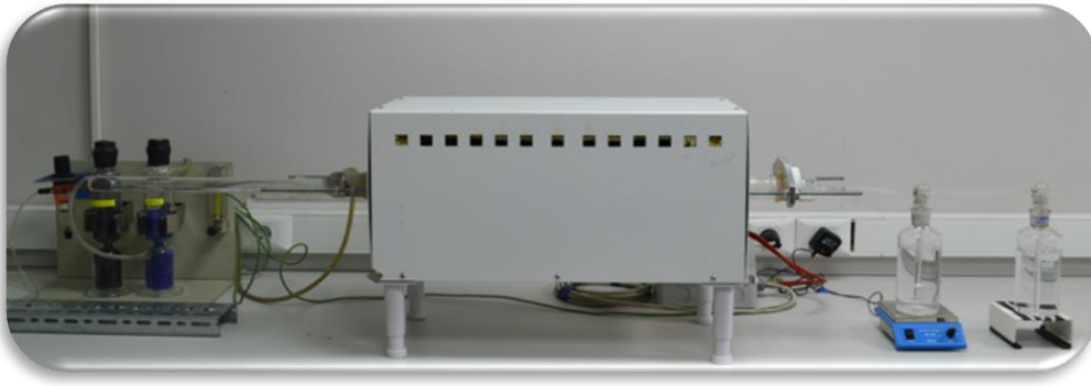
Image 5: EN 60754-2 / Determination of Gas (Ph and Conductivity)
