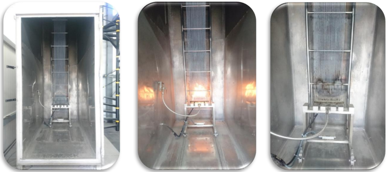
Image 2: View of the tested sample on the ladder (EN 50399)
