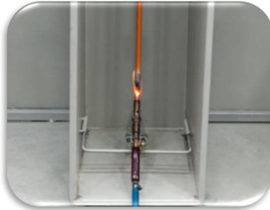
Image 3: EN 60332-1-2 / Vertical Flame Spread Test
